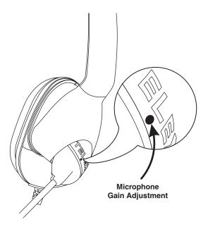
Figure 4: Microphone Gain Adjustment
